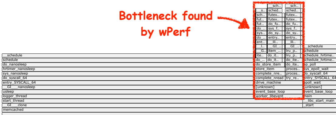
Figure 20: Off-CPU flame graph of Memcached.
